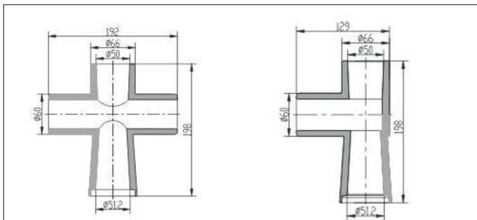
1. The straight and bend bus-bar combined with un-screened crossing connector, bus-bar connector and installed on the socket of the switch.
